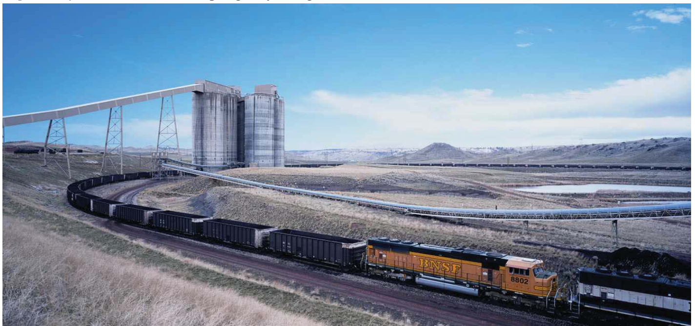
Unit train loading from a Powder River basin mine
