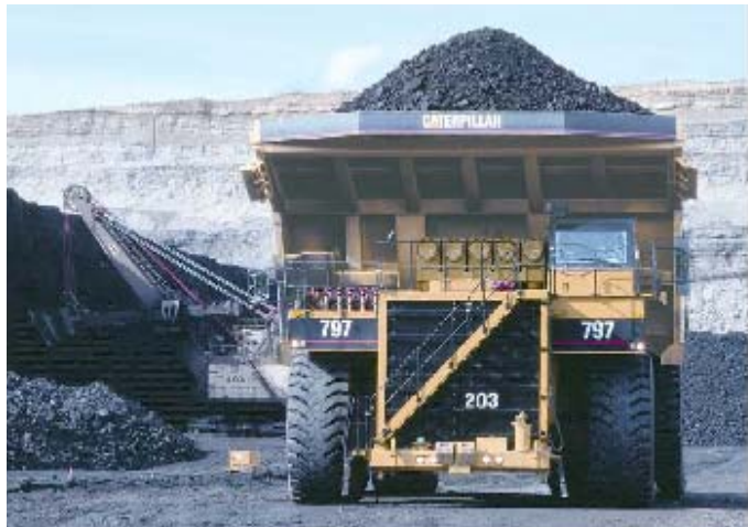
400 ton capacity coal truck
